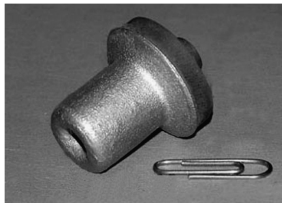
Fig. 12. AlN ceramic detail metallized with Sn–Ti.
